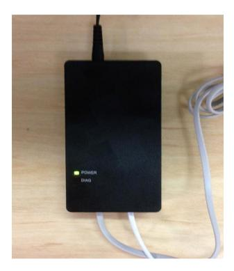
When the connection is working normally the power light should be green and the diagnostic light will be off.
